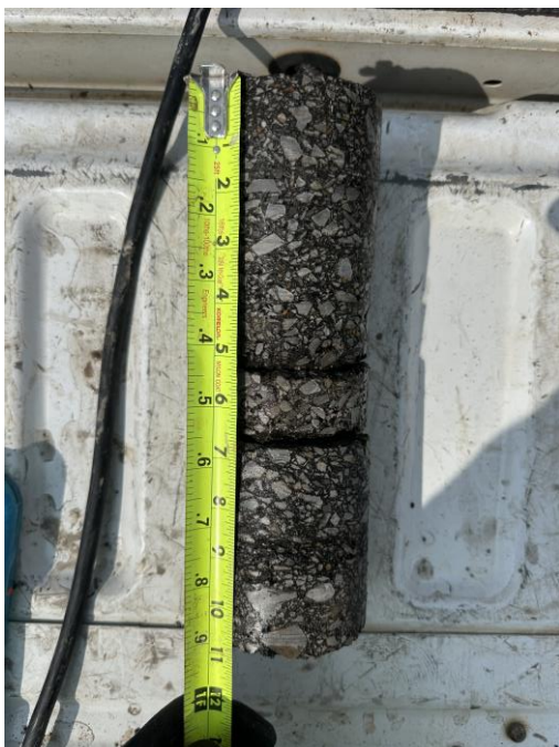
Asphalt Core C-07
